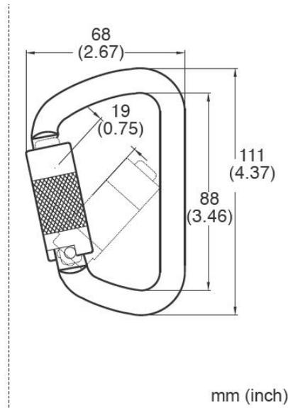
B-Safe BSK0003-16 surpasses current AS/NZS1891.1 (2007) requirements with higher spine and gate capacity –
